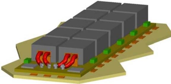
The components of the SCPC could be directly installed on the motherboard, but there are advantages to using a separate daughterboard. All of the fine pitch connections for the solder bumps are confined to the small daughter board, and the entire circuit can be tested before assembly.
