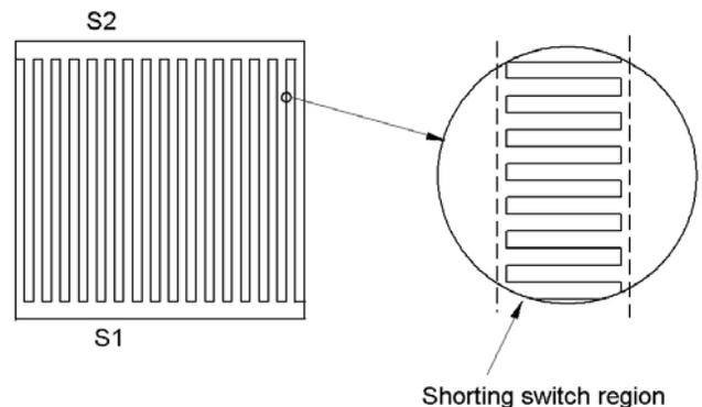
require no connection. However, they must be isolated from the other circuits, so there is an isolation barrier under the area occupied by the shorting switch.
