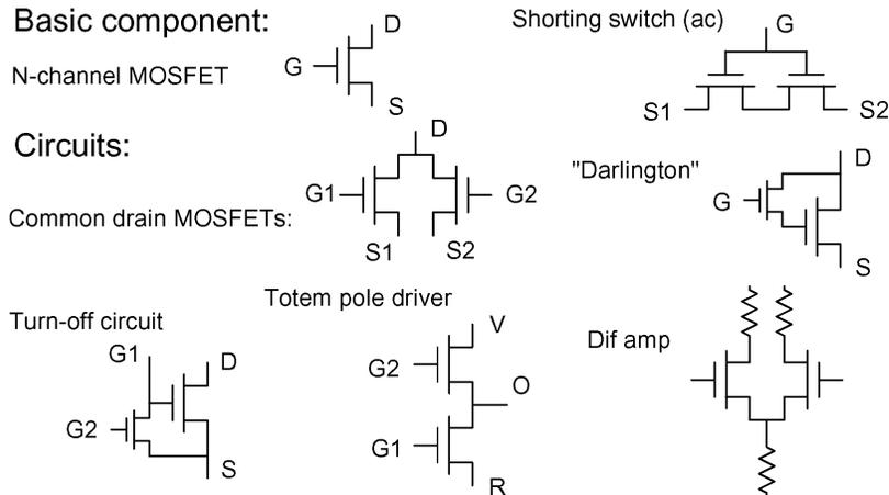
With resistors, many more circuits based upon the old RTL integrated circuit logic family (from the 1960's) can be made, by substituting n-channel MOSFETs for the NPN bipolar transistors.
