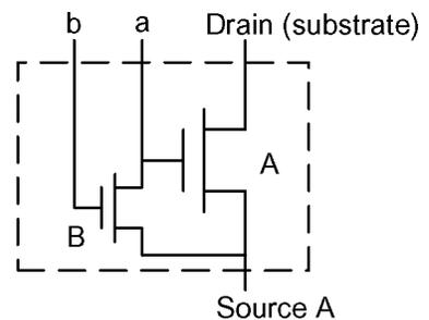
The MOSFETs "A" and "B" are the same except for their active area, and are made at the same time using the same manufacturing processing steps.
