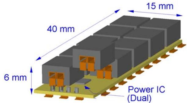
In the module shown, one of the transformer cores is lifted, to show the power IC under the transformers on the daughter board. Components can also be placed on the under side of the daughterboard.
