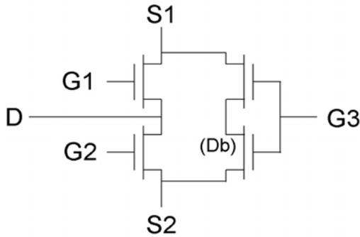
Both of the synchronous rectifier MOSFETs share the common drain connection D, but their sources S1 and S2 and gates G1 and G2 are separate. If the sources are interdigitated, with a pitch P that is small compared to the die thickness L, the area of the drain D is shared and the current density at the drain is halved. High frequency effects are minimized.
